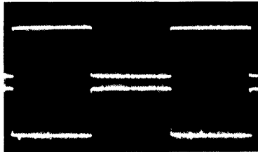
Fig. 7a. Usual appearance of two square-waves without overlap removal
